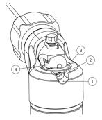
The stroke of the Spektra Edge is adjustable to 2.8mm, 3.5mm, and 4.25mm lengths with the ability to fine tune in between.
